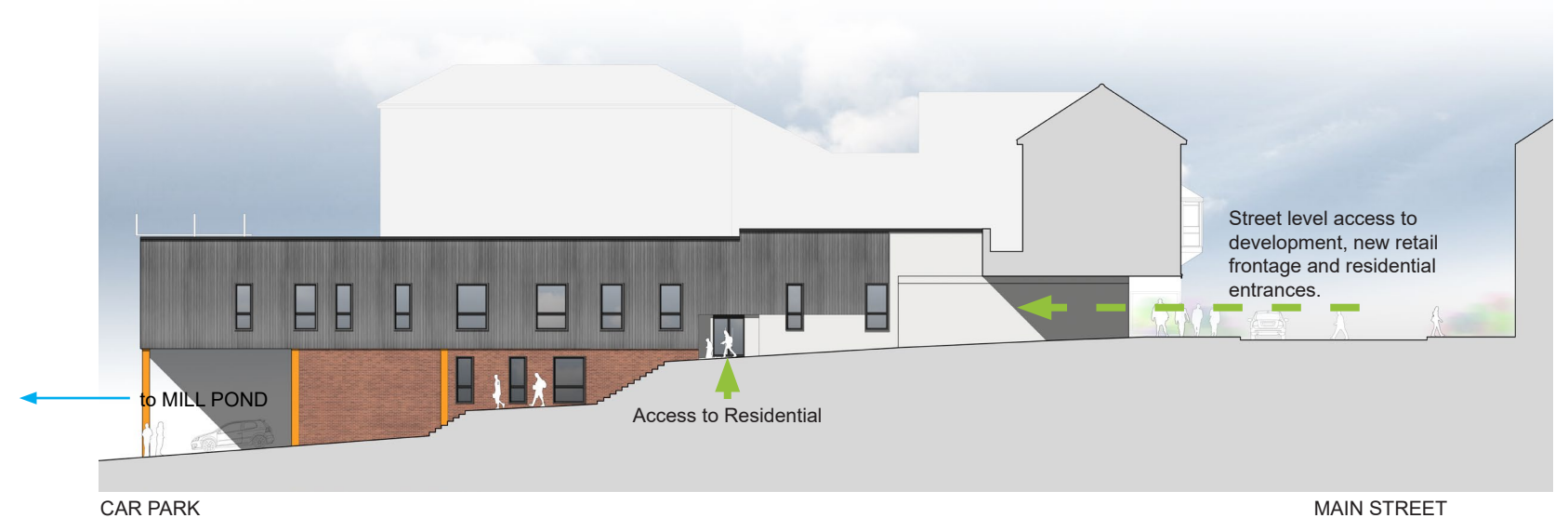
Proposed West Elevation - Level access provided from the High Street and Car Park
