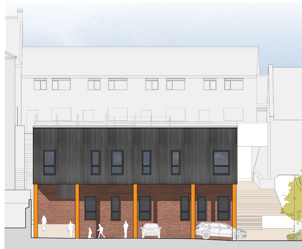
Proposed North Elevation - New full height glazing and coloured columns
